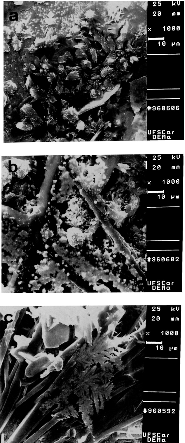
Fig. 11. SEM micrographs for lead films ( v=10 mV/s) obtained from -0.3 V to various potentials as in Fig. 1: (a) -0.73 V; (b) -0.769 V; (c) -1.05 V. Electrolytic solution: 0.100 M Pb(NO_3)_2 + 2.0 M NaOH.
